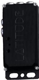
The latitude MDR has wifi connectivity and can be used on DSMC1 and DSMC2 brains to connect foolcontrol to the camera's CTRL port. Latitude system offers advanced features for lens control (internal or external motors, thumbwheels, hand unit...).
